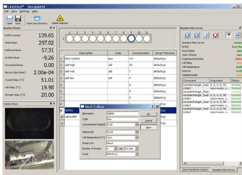
Figure 2 Beamline Experiment Control User Interface. Sample details and wellplate in the center, beamline monitors and cameras to the left, automation control to the right.
